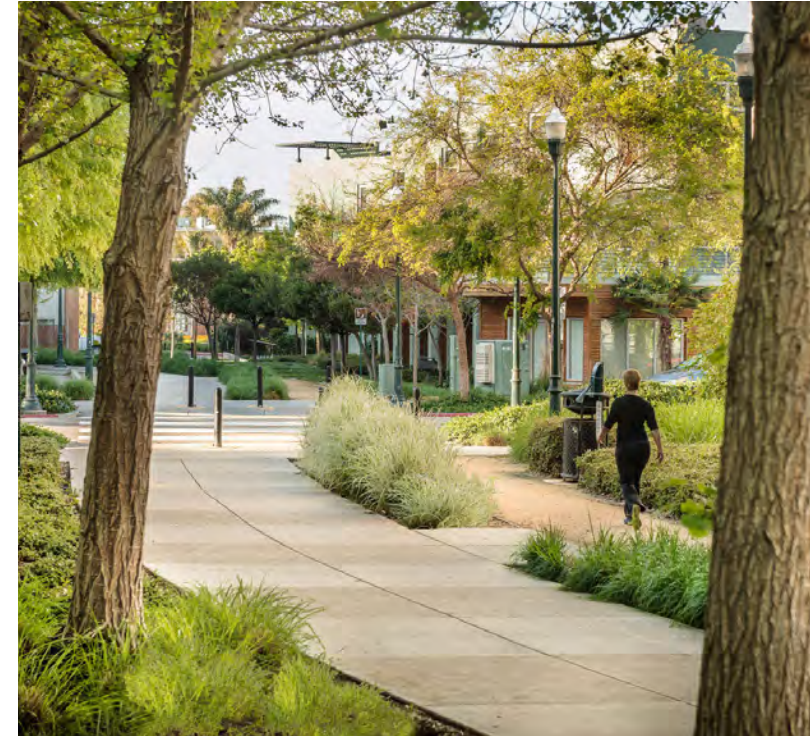
An example of a planting buffer that helps control trail user speed while providing an alternative path of travel for corridor users
